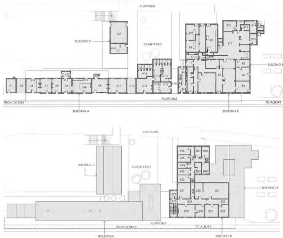
Figure 4-5: Diagram indicating the key buildings. The top panel shows the ground floor arrangement and the bottom panel the first floor (OCP Architects, 2020a:59)
