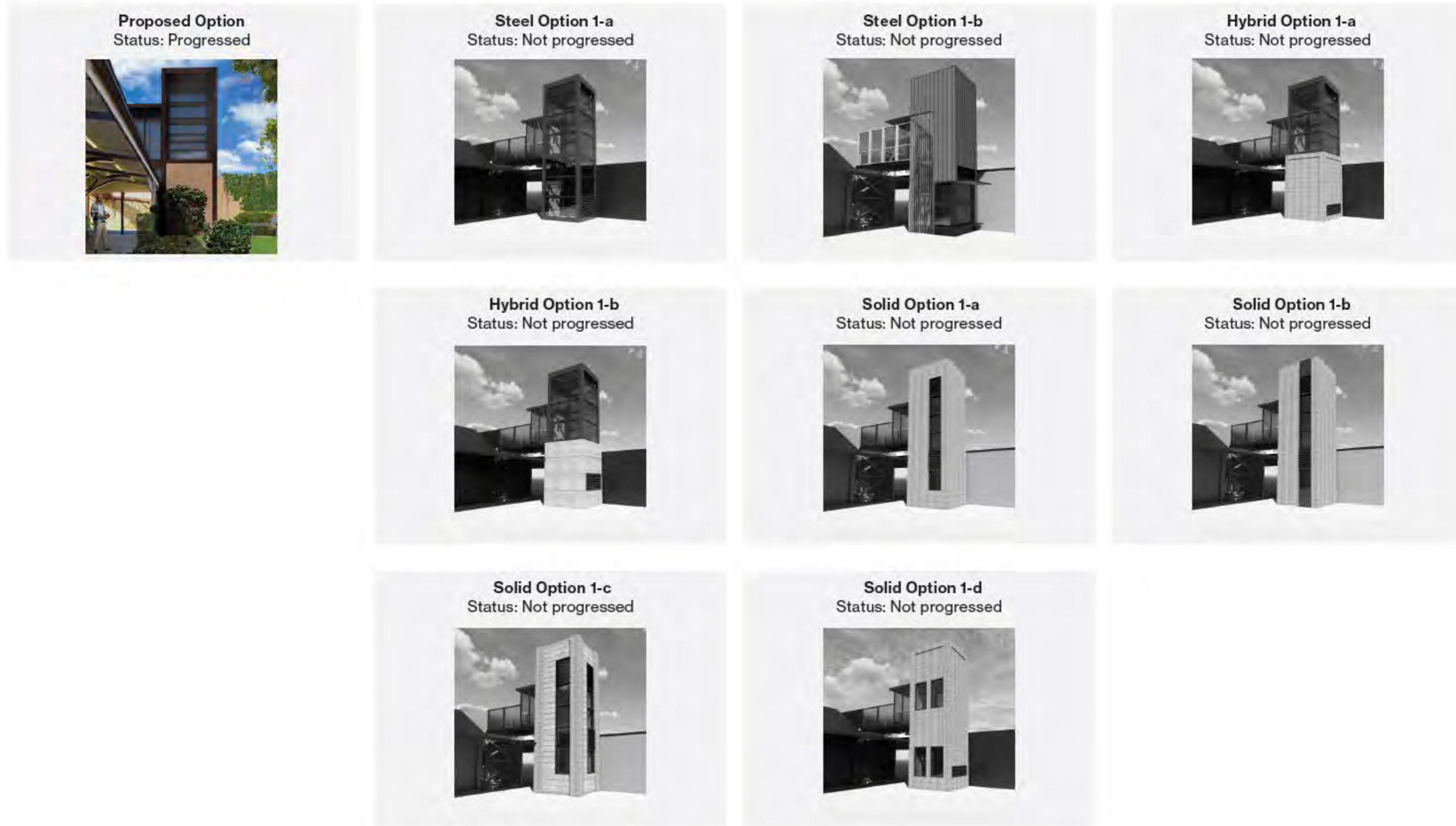
Figure 10.3 Design optioneering for materiality, colour and detailing of the proposed lifts along the Argyle Street footbridge. (Source: Architectus, August 2023)
