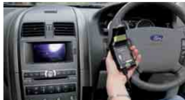
The alcohol interlock device prevents motorists from starting their car if their blood alcohol concentration exceeds 0.02.
