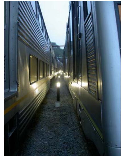
Undesirable narrow track centres at Gosford Yard
